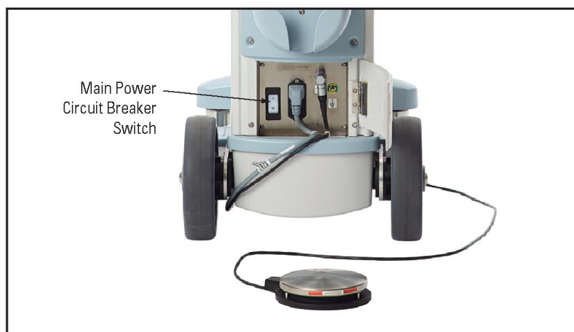
Main Power Circuit Breaker Switch
