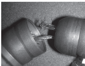
Figure 4 – Appearance of a fraying cable – DO NOT USE
