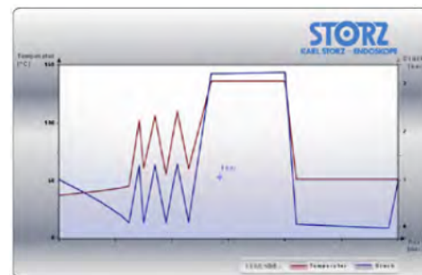
Chronological pressure and temperature profile of a fractionated prevacuum procedure
